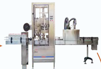
Shrink Sleeve Applicator With Shrink Tunnel
